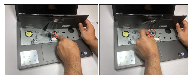
Once the keyboard has been lifted you will notice two conductive tape cables. one large and one small.
