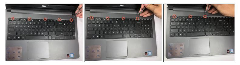
• Use the metal spudger to pry the keyboard off. Do this by inserting the spudger into each of the five indicated slots at the top of the keyboard and gently pulling up on the keyboard with the spudger. Do not be afraid to use a bit of muscle to remove the keyboard, as it takes a bit of force to remove
