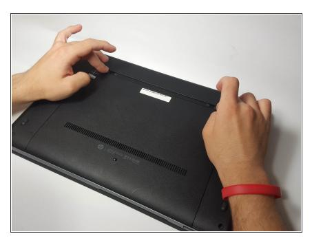
Slide the two battery release latches towards the center of the laptop to release the battery.
