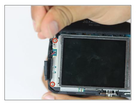
Remove the two 6mm Phillips #000 screws.
