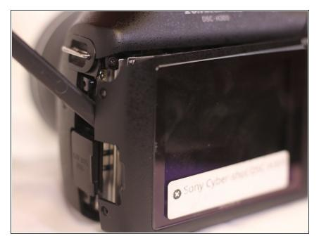
Use the flat end of a plastic spudger to pry apart the rear cover from the body of the camera.
