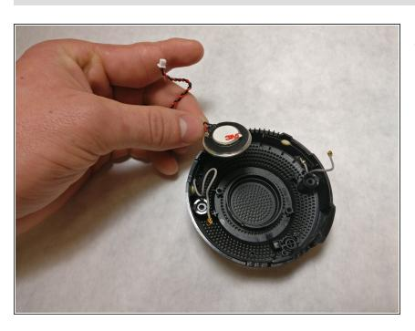
Remove the speaker by gently pulling on the wire near the speaker.
