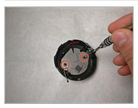
Remove the two 7.25 mm screws using the Ph00 head.
