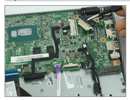
Disconnect the display cable from the motherboard.
