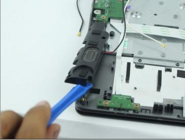
• Remove the speakers located on both left and right bottom corners of the Chromebook with a plastic opening tool.
