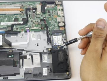
• Remove the 3.6 mm Phillips screw that secures the SSD in place.
