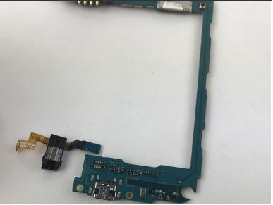
Use the flat end of a spudger to pry up the headphone jack cable connector from its socket on the motherboard.
