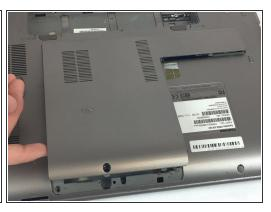
• Use a plastic opening tool to lift up the cover and remove by hand.
