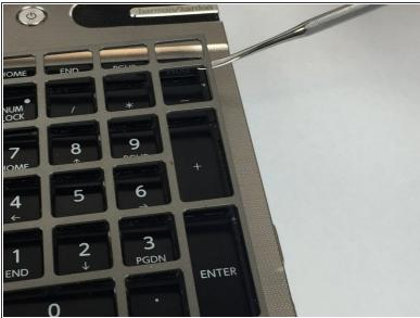
Use a plastic opening tool to pry up the keyboard cover.
