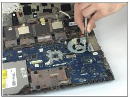
Remove the three 3mm Phillips #0 screws from the fan.
