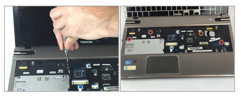
• Remove the four 3mm Phillips #0 screws found underneath the keyboard.
