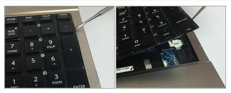
Use a plastic opening tool to pry up the keyboard.
