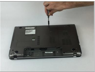
Remove the 3mm Phillips #0 screw from the cover.
