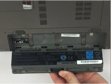
Pull up on the battery to remove.
