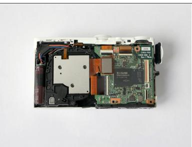
Remove the screws maintaining the last metal protection.
