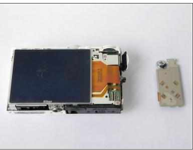
With a plastic spudger, open the ZIF connector and release the button block. It opens from the right side - the black part is to be gently lifted up.
