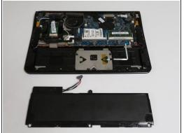
Remove the battery and place it from the laptop. At this point you can replace the battery with a new one.
