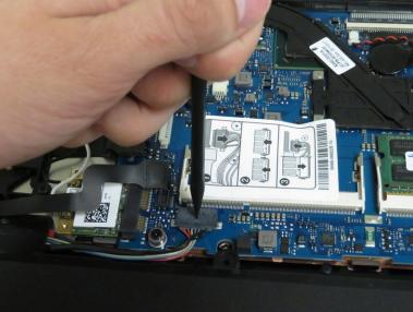
Find the battery's output plug, and use a spudger or pointed precision tool to press on the indention in the middle of the plug to unlock.
