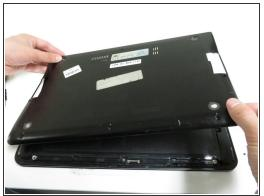
Find an opening on the back of the laptop. Use the plastic prying tool to help pry open the back panel of the laptop.
