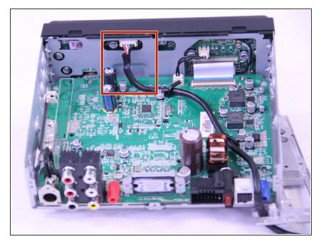
Disconnect the USB cable from the display board.
