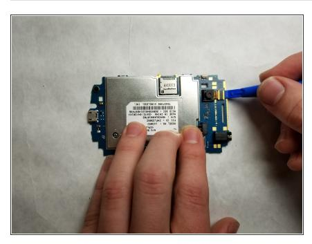
Pry the camera from the internal circuit board with the plastic opening tool and remove it.
