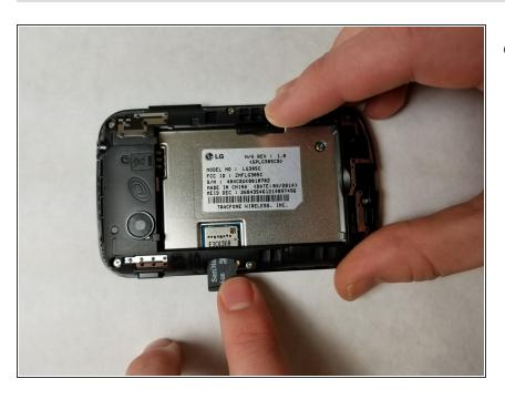
Dislodge the microSD card from the microSD card slot using your index finger and remove it.
