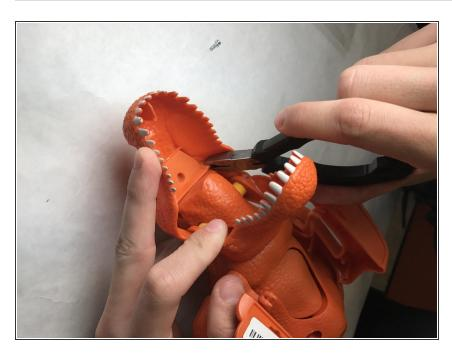
Using tweezers or wire cutters for tension, remove the cover to reveal the LED assembly.
