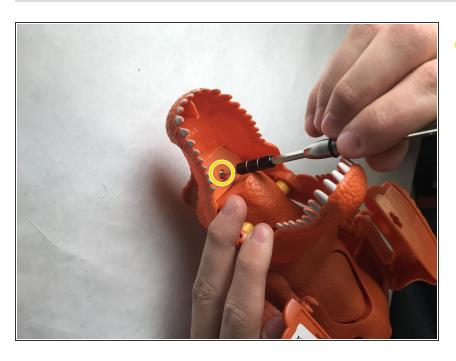
Using a JIS #1 screwdriver, remove the 9.6mm screw.
