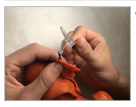
Remove the plastic cover from the top of the LED.
