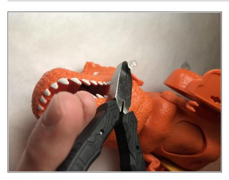
Hold the LED to remove slack from the wires, and cut the wires as shown to remove the faulty LED.
