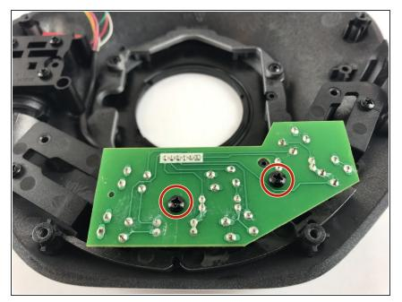
• Remove the two 10mm Phillips #1 screws from the button board.
