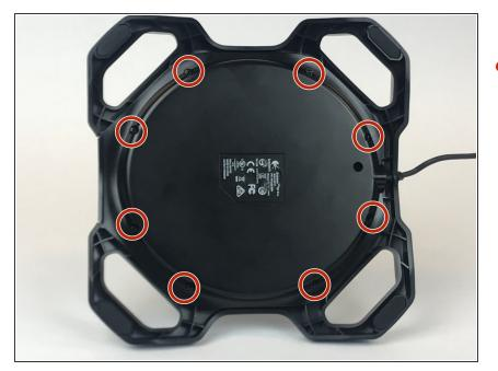
Remove the eight 10mm Phillips #1 screws from the bottom.
