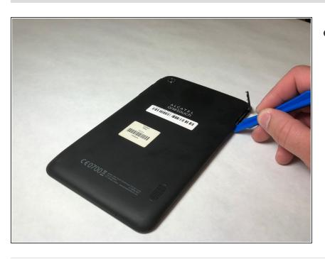
Use the plastic opening tool to pry around the edges of the back cover until it pops off.
