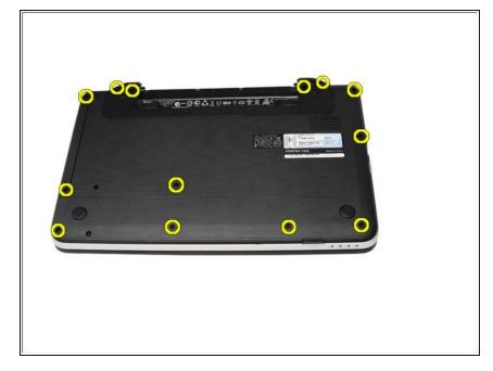
Remove the screws that secure the bottom base.
