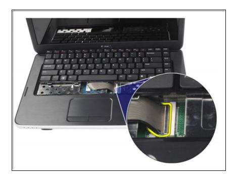
Disconnect the keyboard cable from the system board.
