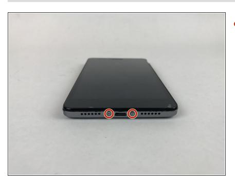
Remove the two 1.17mm Torx T3 screws from the bottom of the phone.
