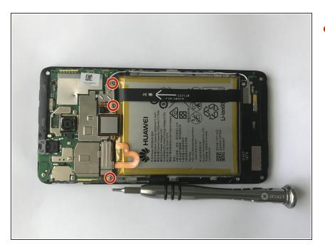
Remove the three 1.5mm Phillips #000 screws.
