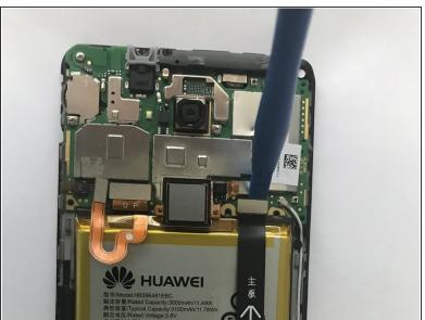
Use a plastic opening tool to disconnect the orange and black battery cables from the motherboard.
