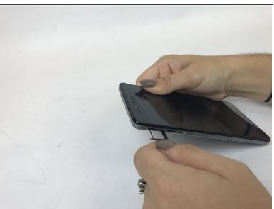
Use the Sim card ejection tool to remove both the sim card trays.
