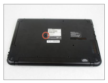
Use a Phillips #1 screwdriver (PH1 bit) to remove the single 7 mm screw that secures the CD/DVD drive.
