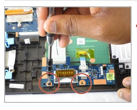
Remove the two 7 mm Phillips screws holding the touchpad component to the back panel using the PH1 bit and Magnetic Driver.
