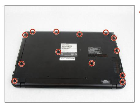
Remove the thirteen 7 mm Phillips screws holding the back cover using the PH1 bit and Magnetic Driver.
