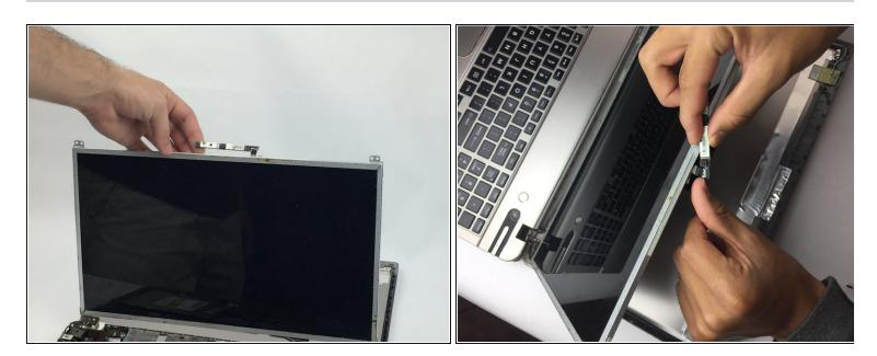
Carefully lift up the screen for an easier removal of the webcam. Then gently remove the connector by sliding it out of the webcam.
