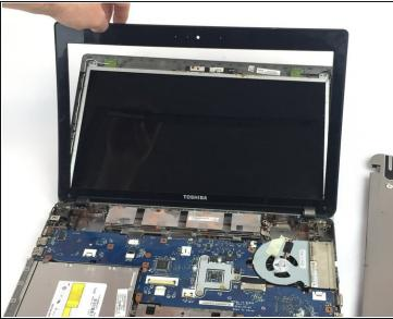
• Using a plastic opening tool, carefully pry open the border of the screen away from the screen until the border is completely off.
