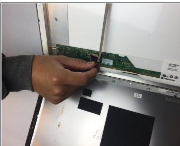
• Remove the tape holding the sliding connector and gently pull it out.
