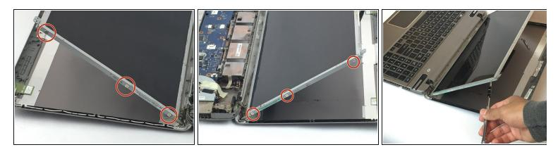
• Using the Phillips 012, remove the three F2 screws on each side of the screen.
