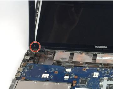
Remove the two F3 screws on the bottom part of the screen.
