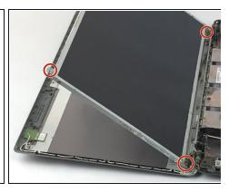
• Using the Phillips 001, carefully remove each F3 screw on each corner of the screen.
