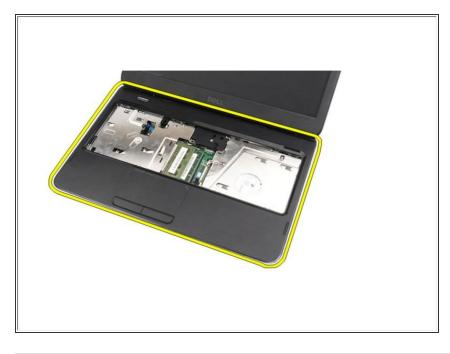
With a plastic carefully pry up the palmrest along the edges. Lift the palm-rest and remove from the computer.
