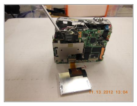
Unthread the four wires running across the top of the viewfinder from the plastic brackets holding them in place.
