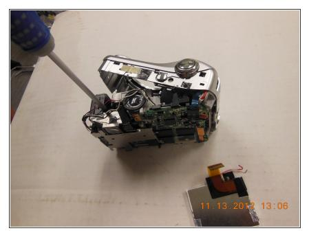
Remove the two black screws threaded vertically into the top of the viewfinder. Loosen the flash and circuit board for more accessibility. This will allow for the viewfinder to be replaced.
