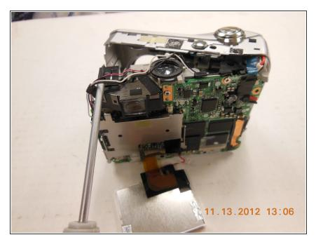
To connect the new screen, solder the wires in place and connect the ribbon cable to the logic board.
