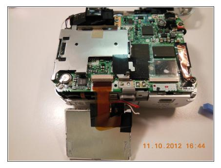
Flip the screen down. To disconnect the ribbon cable from the logic board, rock each end of the brown metal retainer that holds the ribbon cable in place until the ribbon disconnects.
