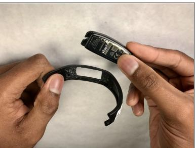
Carefully peel back the wristband so the bottom of the device is facing you. Then, pull out the
