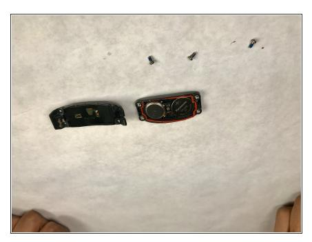
With the screws removed from the device, take the cover off the top of the device, revealing the batteries inside.
