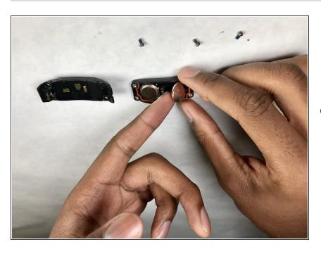
With the cover removed, take out the two batteries currently in the device. Take note of which side of the battery is facing which way in the device. Battery removal can usually be accomplished with your fingers. If not, carefully use a nylon spudger to pull up one edge of the battery, allowing you to remove that battery. To reassemble your device, follow these instructions in reverse order.
