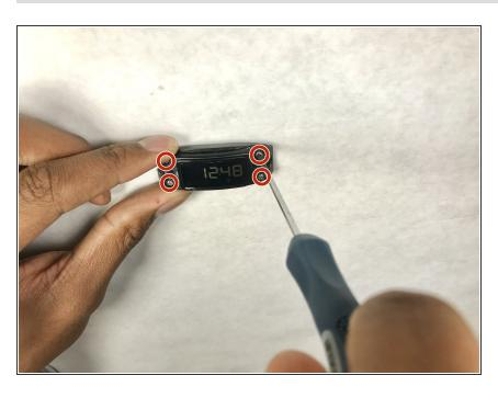
Remove the four 3.8mm Phillips #00 screws holding the device together.
