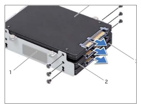
Place the **NEW** primary hard drive (HDD 0) in the hard-drive bracket.
