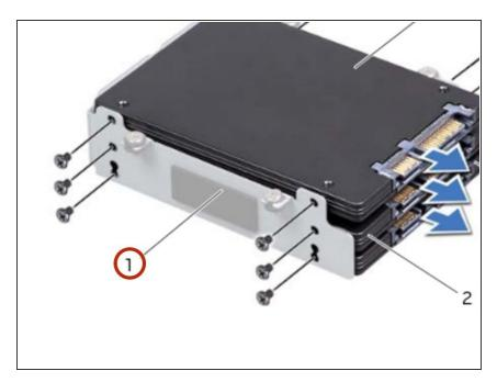
If applicable, slide the secondary and tertiary hard drive(s) into the hard-drive bracket.
