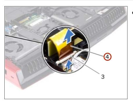
Slide the hard-drive cable into the connector on the system board and press down on the connector latch to secure the cable.
