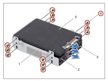
Remove the screws that secure the hard drive(s) and slide the hard drive(s) out of the hard-drive bracket.
