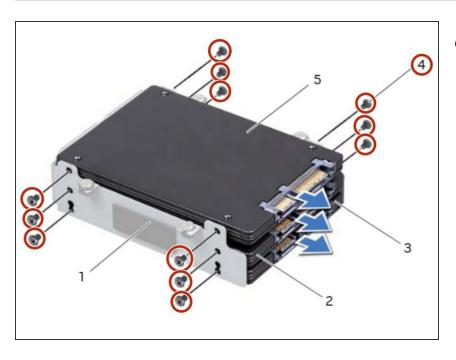
Replace the screws that secure the primary hard drive (HDD 0).
