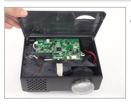
Flip the projector over and then remove the cover by lifting it up.
