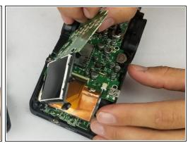
• Unscrew three (PH #1), 7mm screws from the button board near the display and gently flip over.
