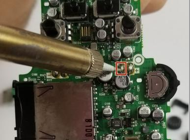
Taking care not to damage other components on the motherboard, use a soldering iron to undo the soldering that holds the terminals to the motherboard.
