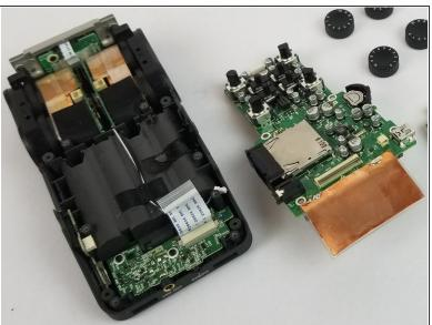
Gently lift off motherboard from the base of the device.
