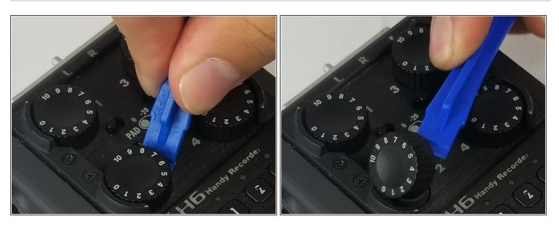
Place device face up and remove the four knobs using the flat end of the plastic opening tool.
