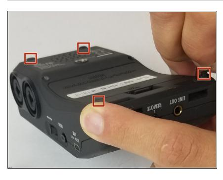
Remove four rubber feet using fingernails to access the four screws underneath.
