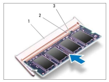
Slide the memory module firmly into the connector at a 45-degree angle, and press the memory module down until it clicks into place. If you do not hear the click, remove the memory module and reinstall it.
