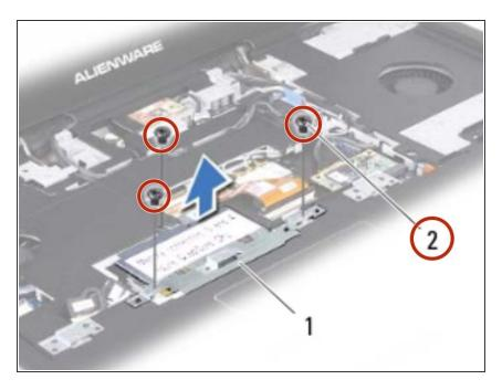
Replace the screws that secure the memory-module cover to the palm rest assembly.
