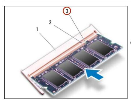
NOTE: If you need to install memory modules in two connectors, install a memory module in the lower
