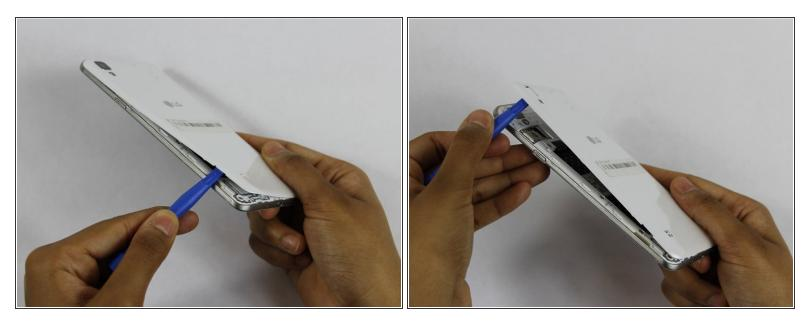
Insert a fingernail, or plastic opening tool, into the cutout on the back cover and pry outward to remove.
