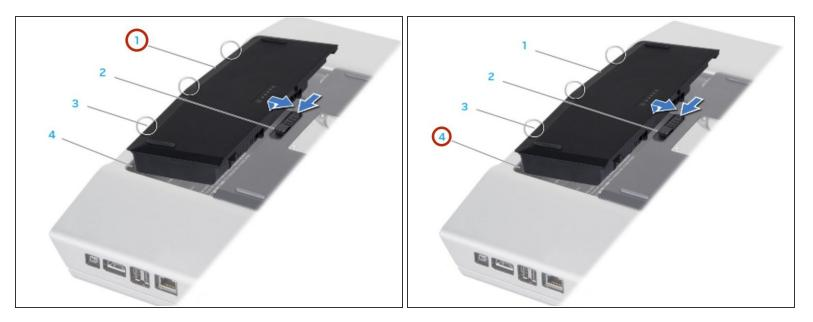
• Slide the battery pack into the battery bay until the battery pack clicks into place.
