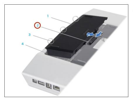
• Slide the battery latch to the unlock position as shown.
