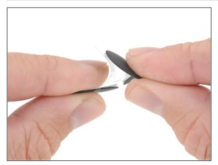
• Peel a replacement foot from the plastic backing.
