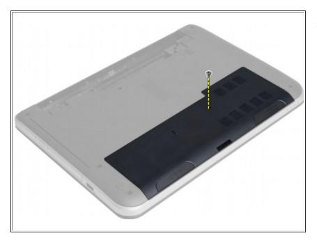
Loosen the screw that secures the access panel and remove it from the computer.
