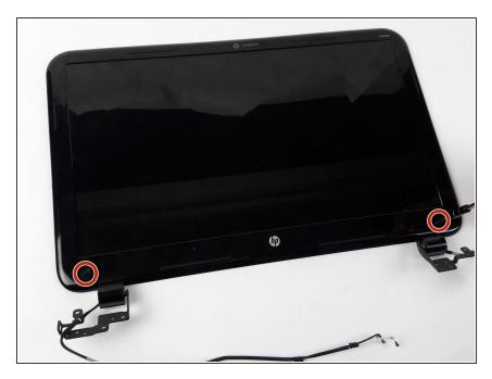
Remove the two 3.5mm Phillips #1 screws from the bottom of the screen.
