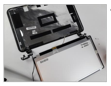
Lay the screen face down on a surface where it ill not scratch
