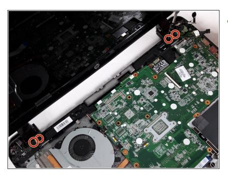
Remove the four 5.5mm Phillips #1 screws attaching the screen.
