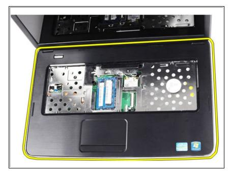
Starting from the left, pry up the palm-rest and remove it from the computer.
