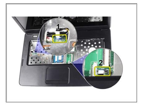
Flip the computer and disconnect the power board cable and the touchpad cable.
