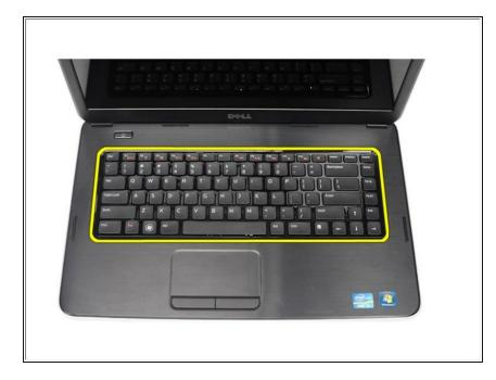
• Flip the keyboard and lay it on the palm-rest.
