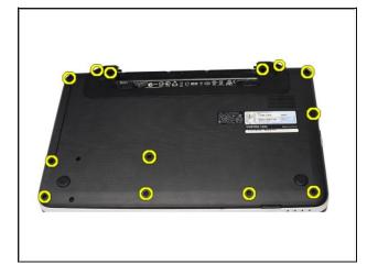
Remove the screws that secure the bottom base.
