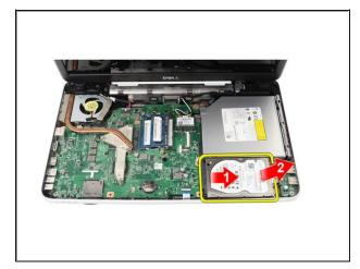
• Slide and lift the hard drive and lift it out of the computer.
