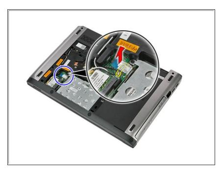
• Disconnect the hard-drive cable from the hard drive.
