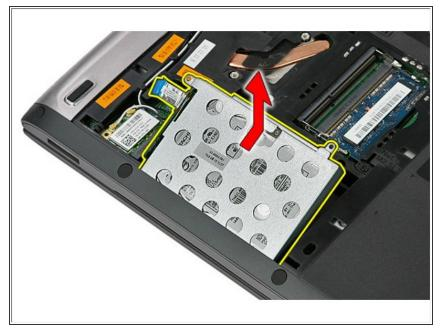
• Lift the hard drive up at an angle from the system and remove it from the computer.
