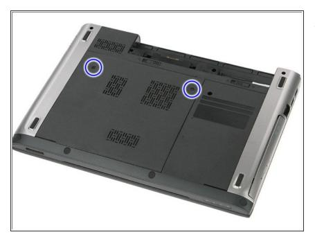
Remove the screws that secures the access panel to the base of the computer.
