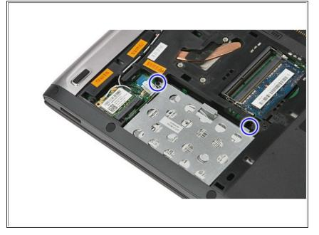
Remove the screws that secure the hard-drive assembly to the computer.
