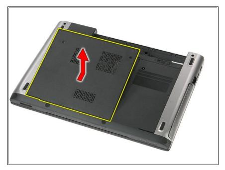
• Lift the access panel up at an angle and remove it from the computer.
