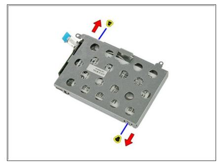
• Remove the screws that secure the hard-drive bracket to the hard drive.
