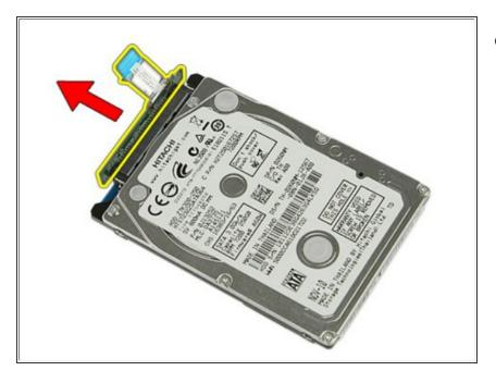
• Remove the hard drive board from the hard drive.
