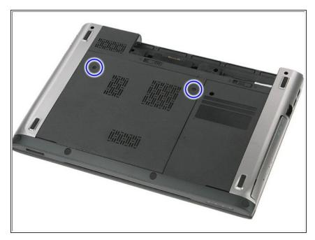
Remove the screws that secures the access panel to the base of the computer.
