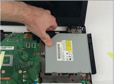
Ensure the screw keeping the disc drive in place is removed, then slide the drive out
