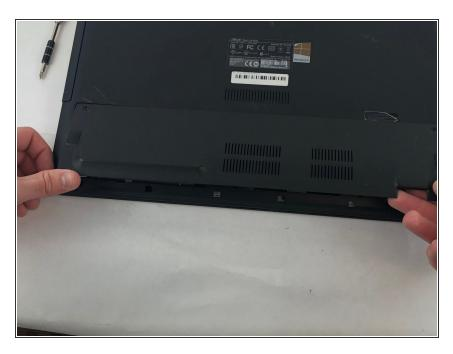
Slide back and remove the protective plating on the back of the laptop.
