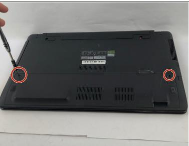
Using the JIS 00 screwdriver, remove the bottom left/right 12.7mm screws located on the back of the laptop.
