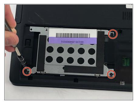
Again with the JIS 00, unscrew the three 5.7mm screws holding the hard drive in place. These can be found on small brackets on the four corners of the drive.
