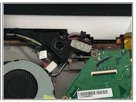
• Remove the wires at the top left of the motherboard, they can just be pulled out
