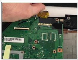
Remove the gold wire from its port by pulling back the tape, then slide it up and out
