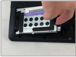
• Slide the hard drive to the left, then remove it by lifting it from the compartment it is resting in.
