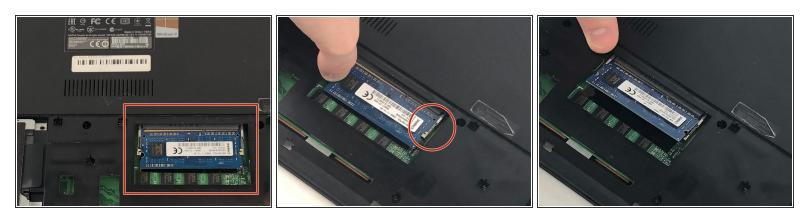
There should be an exposed area located on the right center of the bottom of the revealed compartment. Move the silver brackets holding the RAM to the side. The RAM will pop out of its hold.
