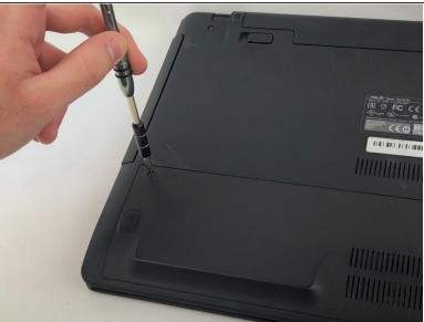
Remove the bottom left and right 12.7mm screws using a JIS 00 screwdriver.
