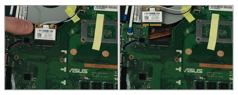
• Disconnect the chip under the fan, connected to the motherboard (you should have removed the screws in step 3)
