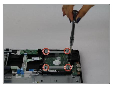
Remove the four 3mm Phillips #0 screws from the hard drive.
