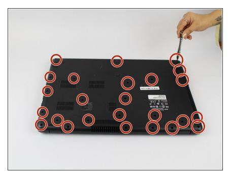
Remove the twenty-five 6mm Phillips #0 screws from the bottom panel of the laptop.
