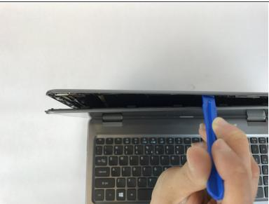
Using a plastic opening tool, pry the back cover away from the screen.
