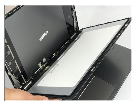
Remove the tape covering the connector cables once the screen is separated from the display board.
