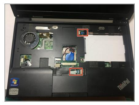
Disconnect the two wired ribbons by pulling up the little black tabs, then pull the wires out.
