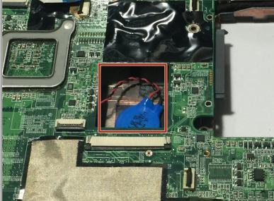
• Simply disconnect the blue connector at the center of the device.
