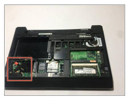
Flip the device back over to untape the two black wires located at the bottom left corner of the device.
