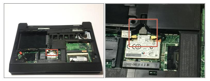
Simply pull the two plugs up and out to disconnect the wires.
