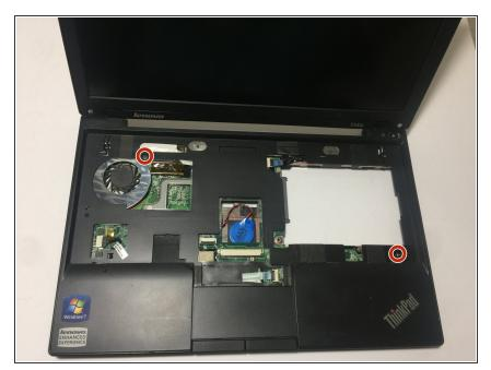
Using the magnetic screwdriver fit with a PH0 bit, unscrew the two screws shown in the picture.
