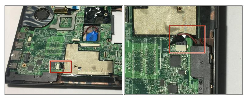
Disconnect the wired plug, then close the device and flip it over.
