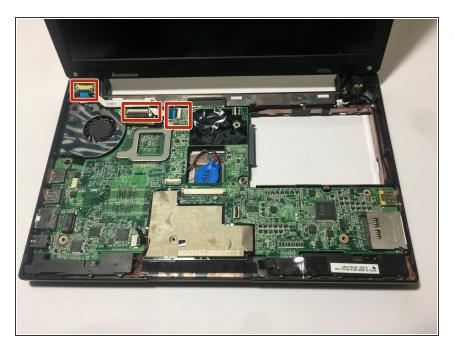
Disconnect the three wired ribbons on the top left side of the panel.
