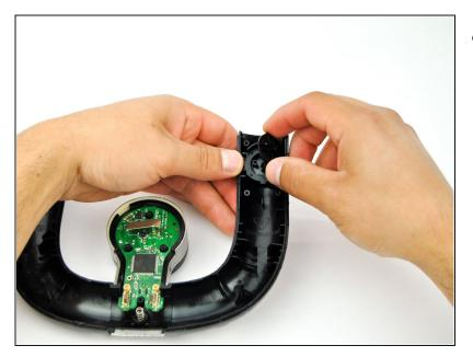
• Lift and remove the black, plastic backing of D-pad. The front of the D-pad will detach as you pull the back off.
