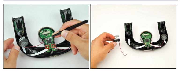
• Use precision tweezers to remove the red and black wires that are attached to the circuit board.
