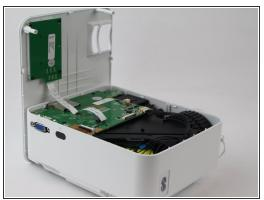
Flip the device over and pry the top off with a plastic opening tool.
