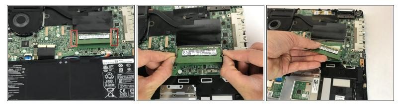
Two clips secure the RAM module in place, one on each side. Using your fingers, spread the clips away from the RAM module.
