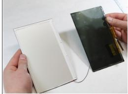
Separate the LCD screen from the metal protecting case with the metal spudger.
