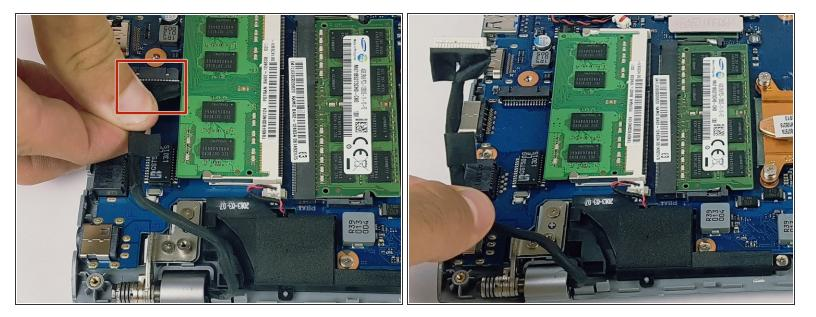
Disconnect the black cable by pulling straight out.
