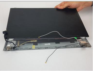
Unscrew the four 3.55mm long screws that hold the display in place.
