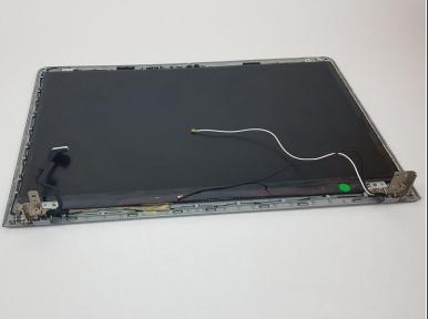
Using the plastic opening tool, pry open the plastic housing that holds the display.
