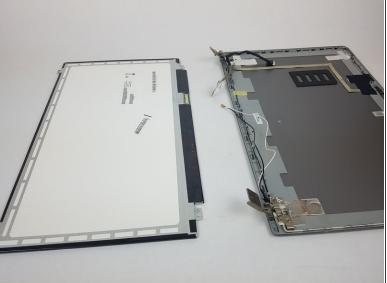
Disconnect the last cable by pulling straight out.
