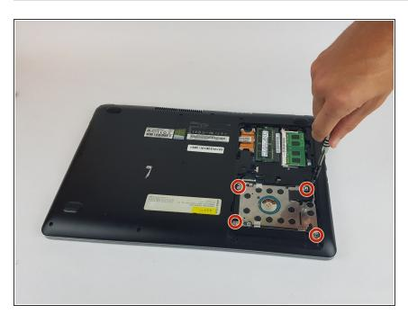
With the cover removed, unscrew all four of the 4.75mm long screws using the Phillips #0 screwdriver.
