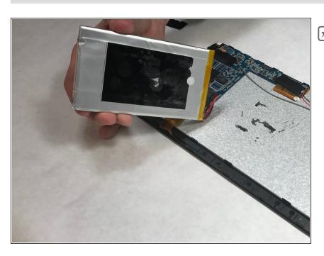
Apply adhesive between the replacement battery and the device before installation.
