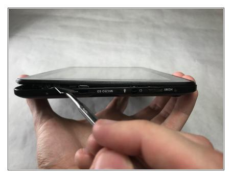
Pry the back cover from the device along the bottom edge.
