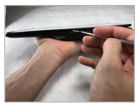
Continue prying along the edge of the device until the back cover is free.
