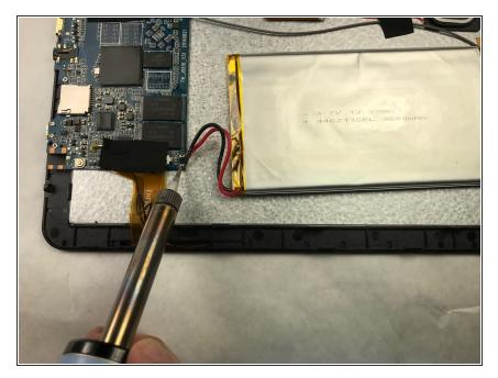
Desolder the faulty battery wires.
