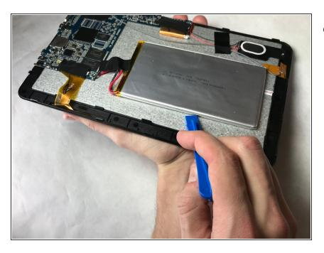
Pry the battery free from the device using a plastic opening tool.
