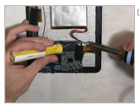
Solder the replacement battery wires to the circuit board.
