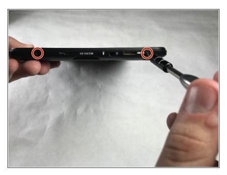
Remove the two 3.2 mm PH000 screws near the charging port.
