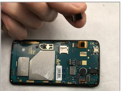
Carefully use the nylon spudger to pry the camera from its connector.
