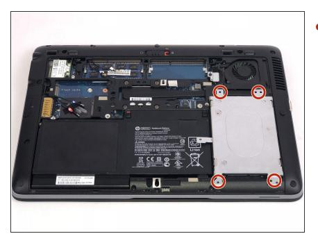
Remove the four 8mm screws with the T7 philip's head.
