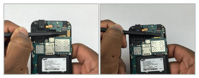
• Using the flat end of a spudger, disconnect the digitizer cable connector.
