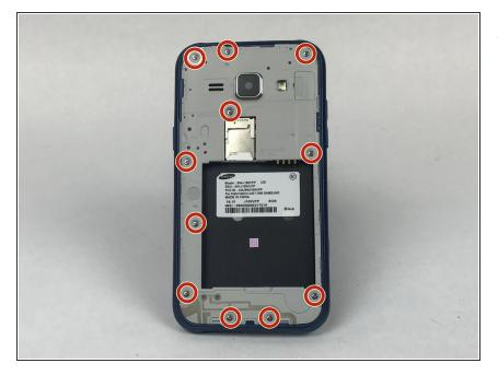
• Using a Phillips #00 screwdriver remove the eleven 3 mm screws.
