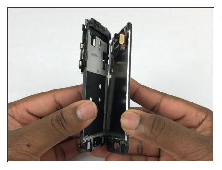
• Carefully separate display assembly from the plastic housing.
