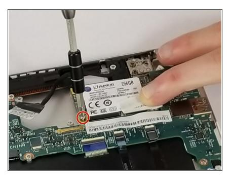
• Remove the marked 2mm screw with a Phillips #01 screwdriver.
