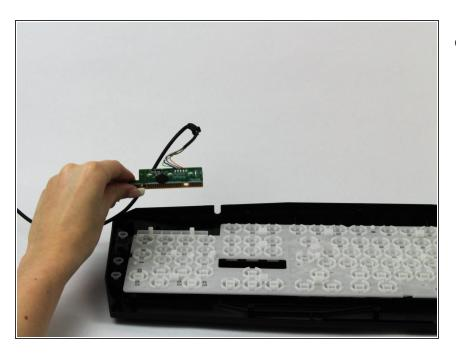
Remove the motherboard and its attached cable from the plastic casing. The cord should now be free and can be replaced.
