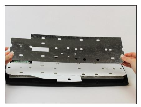
Remove the metal backing located directly underneath the white plastic casing.
