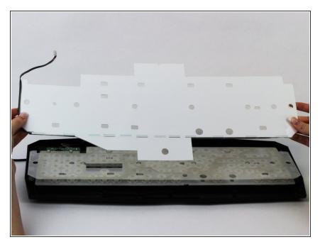
Carefully remove the LED board, which should now come free from the casing.
