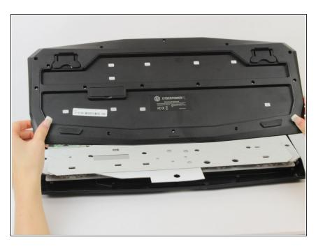
Lift up and remove the plastic casing.
