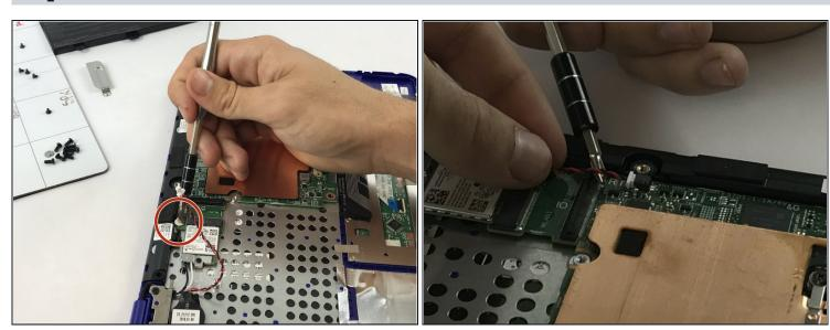
• Remove the 2mm screw that secures the motherboard and keyboard assembly.
