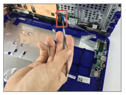
Open the latch and disconnect the I/O-board cable from system board.
