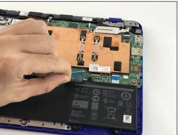
Open the latches and disconnect the touch-pad cable and keyboard cable from the system board.
